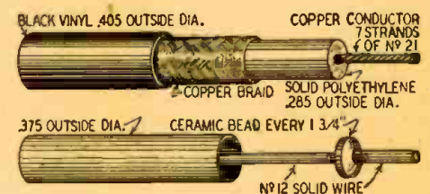
Fig. 6—Two types of popular co-axial cable.
