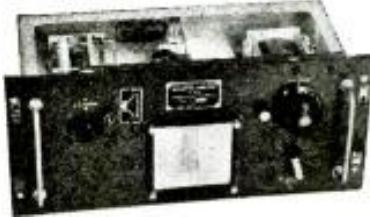
Tuning unit B. C. 375. Each unit has three double spaced tuning cond. Approximately 65 MMFD. Coils 5W chokes national velvet diodes and assorted Mica cond. 2500 WVDC $4.95 over $50.00 in parts.
