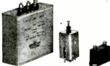
Condenser oil filled, hermetically sealed, 8.5-8.5 M.F.D., 1000 V.D.C., convertible to 4.25 M.F.D., 2000 V.D.C., 5 1/4" long, 2" wide, 5" high. $3.95
