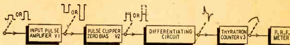
Fig. 2—Incoming wave is first amplified, then clipped and reduced to a sharp pulse.
